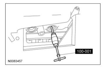
2. NOTE: Oversize plugs are identified by the OS stamped in the flat located on the cup side of the plug.
